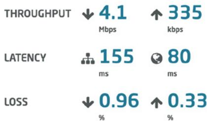
**Throughput:** Every 250ms, ScoreCard measures the upload and download performance of subscriber traffic. Sub-second, frequent measurements provide a better view of application performance than one or five minute averages that most systems collect.
