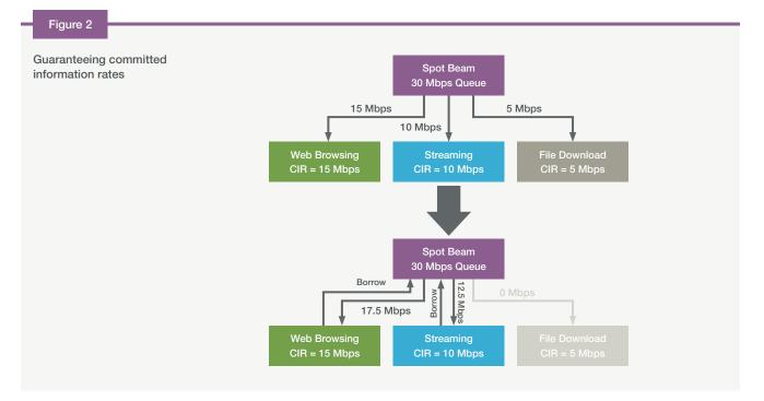
In **Figure 2** (above), bandwidth borrowing allows service providers to implement a series of hierarchical queues, where each child queue is guaranteed a committed information rate. Here the spot beam represents the parent queue, and the child queues represent sub-elements utilizing the beam, such as, an application group, an aircraft, a sea vessel, or end users.
