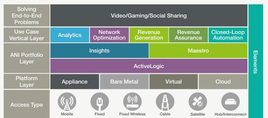
The platform layer of Sandvine's ANI Portfolio consists of bare metal COTS appliances, virtual machines, and cloud. These platforms provide required physical or virtual resources to deliver ANI solutions and use cases.
